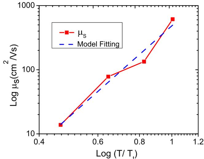
Fig. 6. Electron mobility due to space charge scattering  $\mu_s$  as a function of normalized temperature in log-log scale (red line). Model fitting with (11) (blue dashed line).
