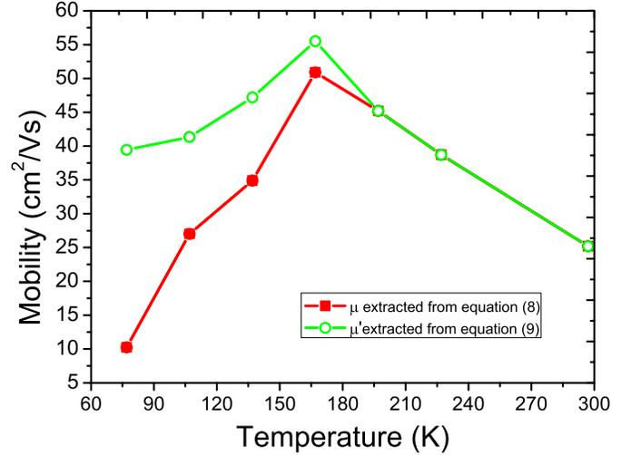
Fig. 5. Extracted carrier mobility in low field region as a function of temperature. The mobility values below  $167$  K are extracted using (8) (red line) and (9) (green line), respectively. The mobility values above  $167$  K are all extracted from (9).
