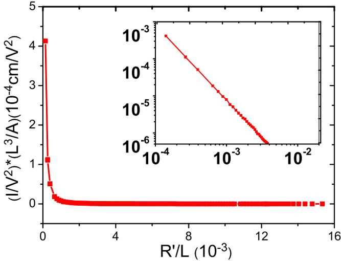
Fig. 4. Scaling behavior for Ti/Au contacted ZnO NW FETs with gate biases ranging from  $-5$  to  $0.8$  V at  $77$  K. The inset is the same data plotted on a log-log scale with a slope close to  $-2$ . The plots show  $(IL^3)/(AV^2)$  follows the scaling relationship  $\xi_0(R'/L)^{-2}$  well.
