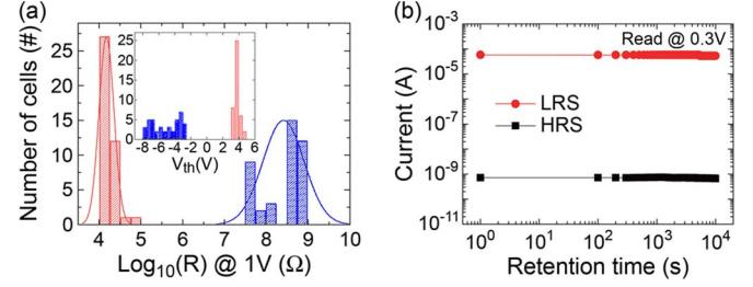
Fig. 2. (a) Histogram of ON and OFF resistance values for P3HT-based organic memory devices. (Inset) Histogram of set and reset threshold voltages. (b) Retention time of the organic memory device.
