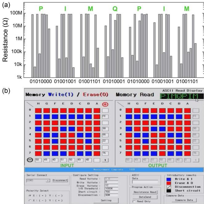
Fig. 4. (a) Logic states of “PIMQPIM” data programmed by the PC-interface memory cell tester. (b) Final image of the demonstration process to address the data into each memory cell with the PC-interface memory cell tester software, showing that the output data are well matched with the input data.
