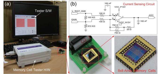
Fig. 3. (a) Optical image of the PC-interface memory cell tester used to independently address the data in the memory cells. At right, two enlarged images show that the organic devices are connected to a package embedded in a socket on a plastic IC chip. (b) Current-sensing circuit to read the resistance state of each memory cell.
