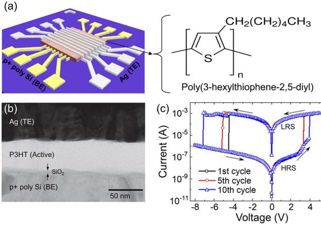
Fig. 1. (a) Schematic of P3HT-based organic memory devices with an  $8 \times 8$  array cell structure. (b) TEM image showing each layer of Ag/P3HT/p<sup>+</sup> poly-Si. (c)  $I$ - $V$  characteristics of an organic memory device.
