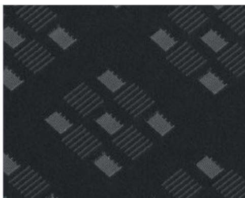
30° tilted SEM image of the lithographically defined InAs nanowires with different diameters and spacings.
