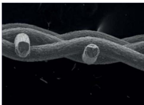
Low-magnification cross section SEM image of TNTs on the Ti-mesh substrate.
