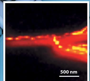
Bundle of carbon nanotubes imaged by tip-enhanced Raman microscopy.
