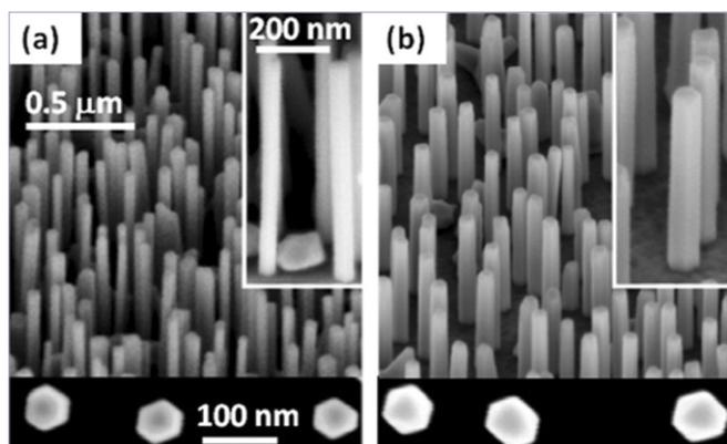
Scanning electron micrographs of InAs nanowires grown on Si(111) at temperatures of (a) 430 °C and (b) 505 °C. Magnified areas (insets) and top-view images (bottom) show the nanowire/substrate interface and hexagonal geometry, respectively.
