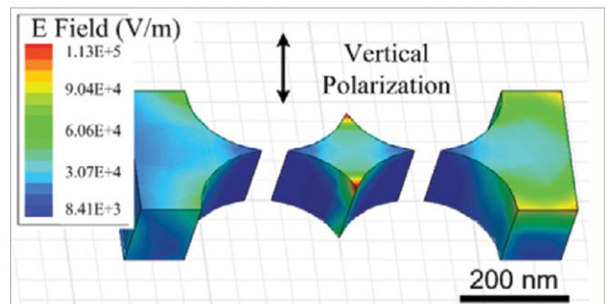
Electrical field distribution within the electrodes with the laser beam polarization normal to the electrode tip pair.
