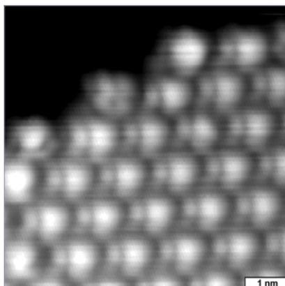
High-resolution scanning tunnelling microscopy image of C60 spray coated on Au(111) at 5 K obtained with the scanning tunnelling parameters:  $U = 2.5$  V and  $I = 85$  pA.
