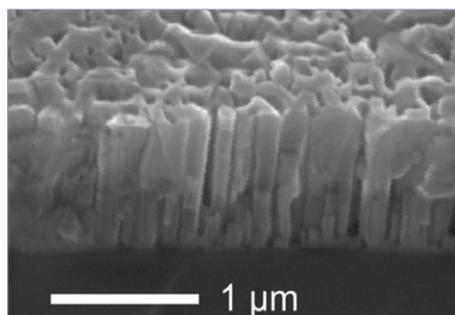
Scanning electron microscopy image showing a continuous GaN:Mg top contact layer grown on GaN nanowires.
