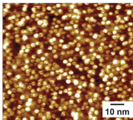
NC-AFM image of Ni deposited at room temperature on the clean  $\alpha\text{-Al}_2\text{O}_3(0001)$  surface.
