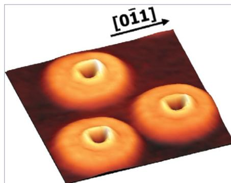
480×480 nm atomic force microscopy image of a typical CRD.
