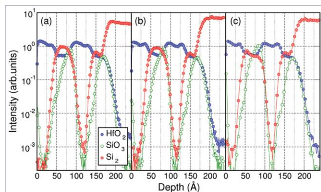
ToF-SIMS profile of the  $\text{HfO}_2/4\text{ nm thick SiO}_2/\text{HfO}_2$  multilayer structure without  $\text{SiO}_2$  capping layer before (a) and after thermal treatment at 600 °C (b) and 900 °C (c) in  $\text{N}_2$  atmosphere for 60 min. The intensity of the  $\text{Si}_2$  signal at the surface increases with the annealing temperature.
