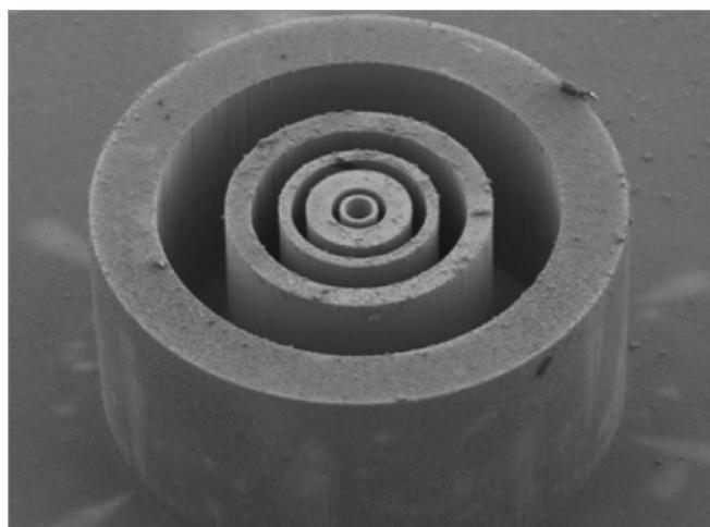
Scanning electron microscopy image of three-dimensional microstructures etched in silicon covered with nickel-coated TMV.
