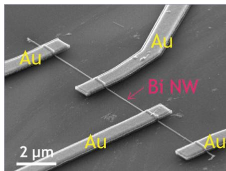
Scanning electron microscopy image of four-probe device based on an individual Bi nanowire to investigate its transport properties.
