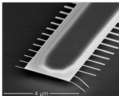
Series of freestanding cantilevers on (100) Si substrate. The implantation dose was  $4 \times 10^{15}$  ions cm<sup>-2</sup>. The length of the cantilevers is 0.5  $\mu\text{m}$  (left) and 1  $\mu\text{m}$  (right), the thickness approx. 50 nm and the width of the narrowest beams 35 nm. The two bridges adhere to the substrate because of stiction deriving from the drying step of the wet release process.
