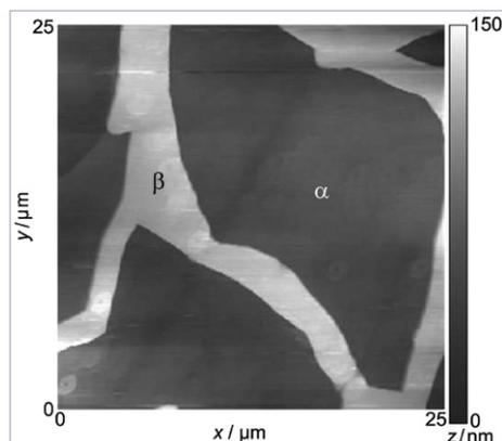
SECM–SFM topographical image of a coarse-grained Ti-6Al-4V specimen in a solution of 2 mM  $[\text{Ru}(\text{NH}_3)_6]\text{Cl}_3$  in 0.1 M KCl. The image was scanned from right to left.
