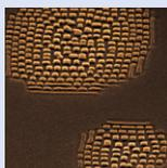
Nanoisland pattern transfer to polydimethylsiloxane (PDMS) taken from the article 'Nanoimprinting using self-assembled ceramic nanoislands' by **Lawrence Burr Zimmerman, M D Rauscher, J Ellis, P Boukany and L James Lee** 2010 *Nanotechnology* **21** 045304
