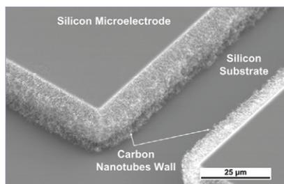
Scanning electron microscopy image of the silicon microelectrode, silicon substrate, and CNT wall.
