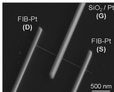
Scanning electron microscopy image of an enhancement-mode FET device on a ZnO nanowire. The source [S] and drain [D] electrodes were fabricated by FIB-deposited Pt, while the gate [G] Pt electrode is lying on an *in situ* deposited SiO<sub>2</sub> layer on the ZnO nanowire surface.
