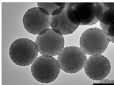
Transmission electron microscopy image showing gold shell growth using LPS@C18N3@Au seed.
