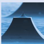
SEM image showing a completed silicon chip made via the microfabrication process taken from the article 'Fabrication of co-axial field emitter tips for scanning probe energy loss spectroscopy' by **Mi Yeon Song, Alex P G Robinson and Richard E Palmer** 2010 *Nanotechnology* **21** 155304
