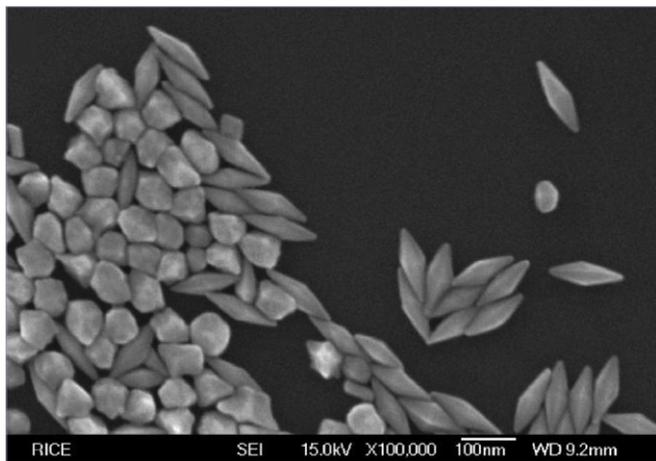
Scanning electron microscopy image showing gold bipyramid structure.
