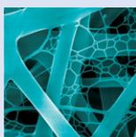
FE-SEM image of PAA fibrous membrane taken from the article 'A highly sensitive humidity sensor based on a nanofibrous membrane coated quartz crystal microbalance' by **Xianfeng Wang, Bin Ding, Jianyong Yu, Moran Wang and Fukui Pan** 2010 *Nanotechnology* **21** 055502
