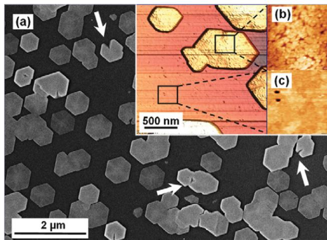
Study of the nucleation seed defects for 100 s nucleation time at 1000 °C without silane flow. (a) scanning electron micrograph showing the hexagonal-shaped seeds and the usual defects indicated by white arrows. The inset shows (b) atomic force microscopy images of seeds (height about 50–200 nm, and 0.8 nm RMS) and (c) in-between the seeds (0.2 nm RMS).
