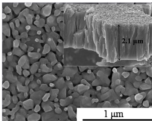
Scanning electron microscopy (SEM) images of WO<sub>3</sub> layers after annealing at 450 °C in air for 1 h followed by a NH<sub>3</sub> treatment at 600 °C. The treatment time is 4 h for all the samples. The inset shows a cross-sectional SEM image.
