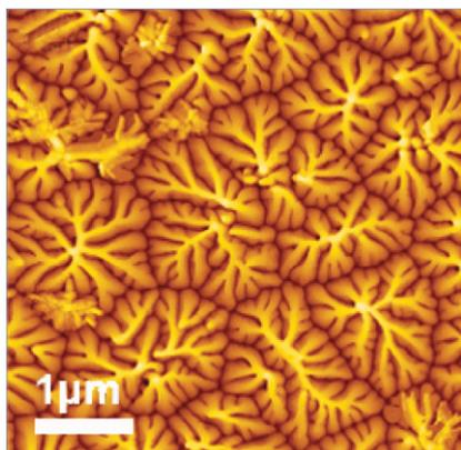
Topographic tapping mode atomic force microscopy image. c-axis-oriented pentacene thin film deposited onto a mica surface kept at RT in a vacuum formed using a diffusion pump with a base pressure of  $5 \times 10^{-5}$  Pa.
