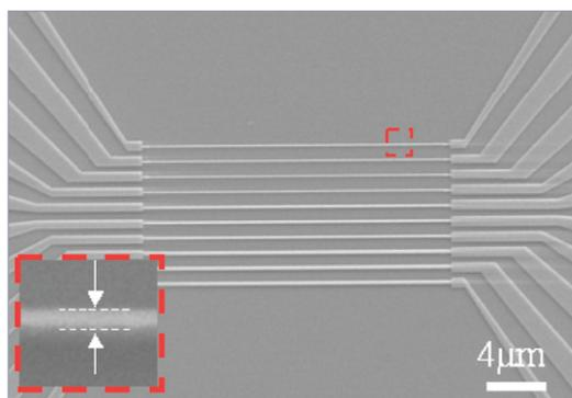
Silicon nanowire sensor arrays fabricated by the top-down nanofabrication process (inset: 50 nm width).
