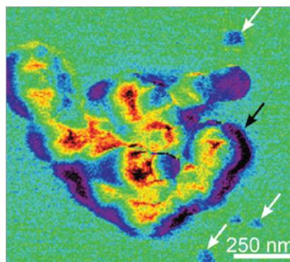
MFM phase shift images at lift heights of 15 nm containing a cluster of  $\text{Fe}_3\text{O}_4$  NPs (black arrow) and scattered AuNPs (some examples with white arrows).
