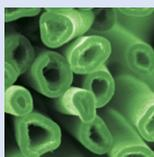
TiO<sub>2</sub> nanotube arrays with Pt nanoparticles, prepared using a bulk technique taken from the article 'Ta<sub>2</sub>O<sub>5</sub>- and TiO<sub>2</sub>-based nanostructures made by atomic layer deposition' by **Marianna Kemell, Emma Härkönen, Viljami Pore, Mikko Ritala and Markku Leskelä** 2010 *Nanotechnology* **21** 035301
