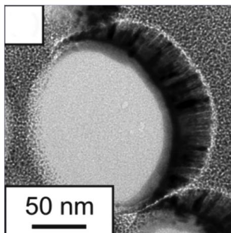
Cross-sectional transmission electron microscopy image of a magnetic cap grown on a 160 nm SiO<sub>2</sub> particle.
