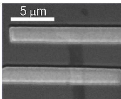
Optical microscope image of a typical FLG device. The scale bar represents 5  $\mu$ m.
