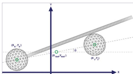
A schematic of the fabricated nanotool is shown. The coordinate system  $(x, y)$  is defined such that the average position of the tool is equal to zero,  $\langle x_{\text{tool}}, y_{\text{tool}}, \theta_{\text{tool}} \rangle = (0, 0, 0)$ . The green circles represent the location of the relevant coordinate, and the subscripts refer to the position of the tool, microsphere 0, or microsphere 1.  $\theta_{\text{tool}}$  is the angle of the tool, relative to the  $x$ -axis.
