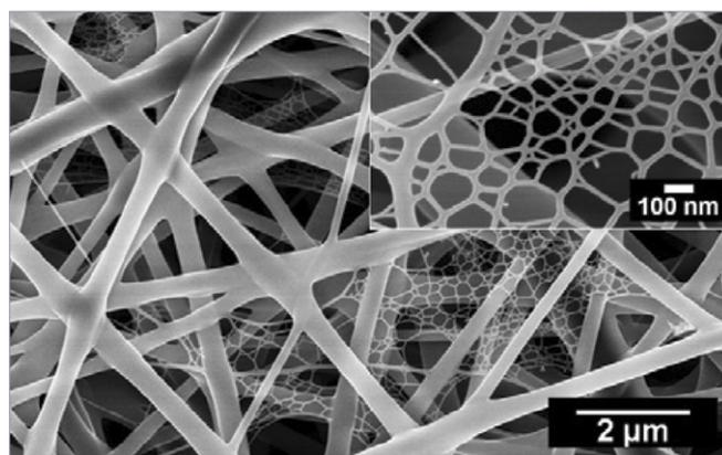
Field-emission scanning electron microscopy images of PAA fibrous membranes.
