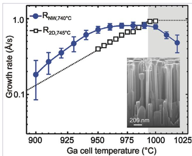
Growth rate comparison between GaN in NWs grown at  $T_{\text{sub}} = 740^\circ\text{C}$  and R2D measured at  $T_{\text{sub}} = 745^\circ\text{C}$  as a function of  $T_{\text{Ga}}$ . The grey shading represents the regime where the impinging Ga flux is higher than the active N flux at  $T_{\text{sub}} = 745^\circ\text{C}$ . The inset is a scanning electron microscopy image of a NW ensemble.
