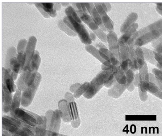
Transmission electron microscopy image of the ZnO nanorod sample  $13 \times 50$  nm synthesized from solution.
