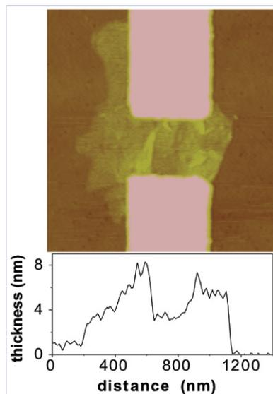
Tapping-mode atomic force microscopy image of an RGO device assembled via DEP along with its height profile. The thickness varies from 2 to 10 nm in the channel, indicating that up to 10 layers of RGO sheets have been assembled in the channel.
