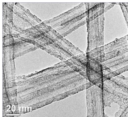
Transmission electron microscopy image of several CNTs covered with a layer of NiO nanoparticles.
