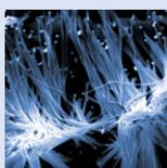
An array of CdTe nanowires taken from the article 'Multisegment CdTe nanowire homojunction photodiode' by **Elena Matei, Lucian Ion, Stefan Antohe, Reinhard Neumann and Ionut Enculescu** 2010 *Nanotechnology* **21** 105202
