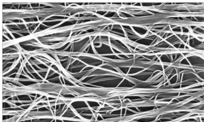
Scanning electron microscopy image of a free-standing MWNT sheet.
