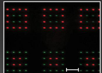
Multiplexing of PEG dot arrays deposited onto a glass slide. Scale bar = 20  $\mu$ m.
