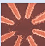
Single-walled nanotubes with diameters that can be tuned in different segments by fast temperature control in laser-assisted chemical vapour deposition taken from the article 'Diameter modulation by fast temperature control in laser-assisted chemical vapor deposition of single-walled carbon nanotubes' by **M Mahjouri-Samani, Y S Zhou, W Xiong, Y Gao, M Mitchell, L Jiang and Y F Lu** 2010 *Nanotechnology* **21** 395601
