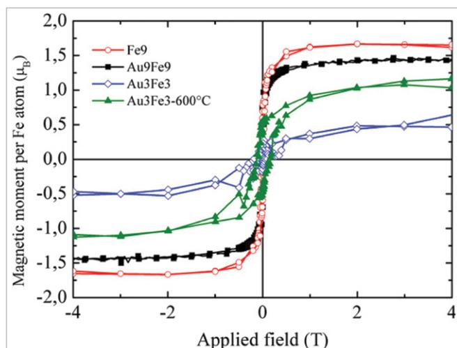
Hysteresis loops measured at 3 K of the Au<sub>9</sub>Fe<sub>9</sub>, Au<sub>3</sub>Fe<sub>3</sub> and Fe<sub>9</sub> as-implanted samples, and of the Au<sub>3</sub>Fe<sub>3</sub> sample after 1 h thermal treatment at 600 °C.
