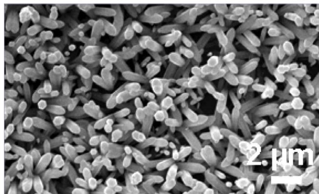
Top-view scanning electron microscopy image of ZnO nanorod array obtained by passing a charge density of 2.5 C cm<sup>-2</sup>.
