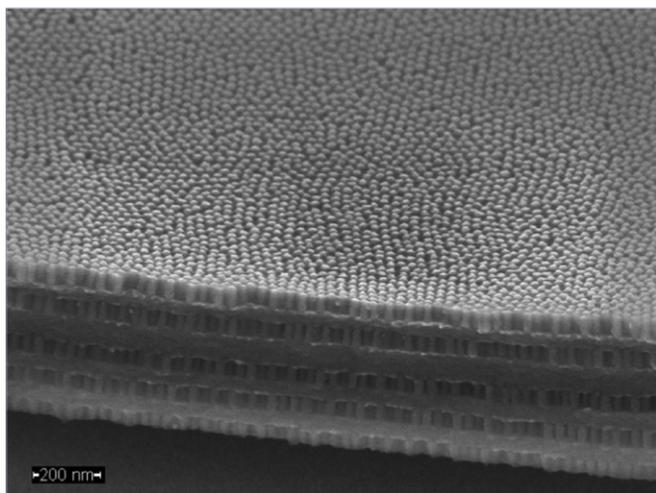
Multi-layer  $\text{TiO}_2$  structure. (Note: The multi-layer structure in the picture was produced accidentally. We are still looking for a method to consistently reproduce the multi-layer structure. But this accident gives strong evidence that the multi-layer structure can be very sturdy and its fabrication is highly possible.)
