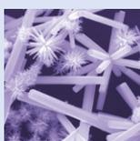
SEM image of ZnO nanorods grown for a seeded hydrothermal mixture taken from the article 'Laser-assisted hydrothermal growth of size-controlled ZnO nanorods for sensing applications' by **S J Henley, J Fryar, K D G I Jayawardena and S R P Silva** 2010 *Nanotechnology* **21** 365502
