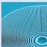
SEM image of 1 μm thick Fresnel zone plates fabricated by electroplating Au in PMMA molds taken from the article 'Direct e-beam writing of dense and high aspect ratio nanostructures in thick layers of PMMA for electroplating' by **Sergey Gorelick, Vitaliy A Guzenko, Joan Vila-Comamala and Christian David** 2010 *Nanotechnology* **21** 295303
