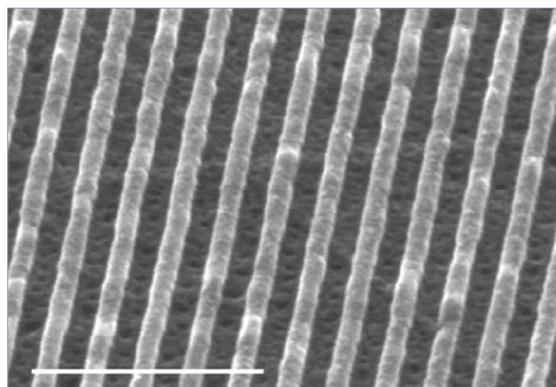
Scanning electron microscopy image of 200 nm period metal gratings in nickel patterned by LADI with a laser fluence of 0.41 J cm<sup>-2</sup>. Scale bar is 1 μm.
