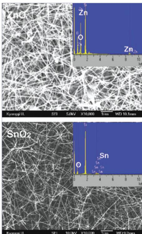
Field-emission scanning electron microscopy images of ZnO nanowires ( $D \sim 70$  nm) and SnO<sub>2</sub> nanowires ( $D \sim 40$  nm). The images in the inset show EDS data for ZnO and SnO<sub>2</sub>.
