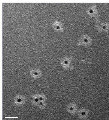
Transmission electron microscopy image of a conjugate of TFG protein and gold nanoparticles. Sample was stained by 3% phosphotungstic acid. Bar size: 20 nm.
