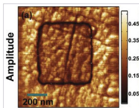
The piezoresponse force microscopy amplitude for a given frequency reconstructed from the simple harmonic oscillator fit parameter.
