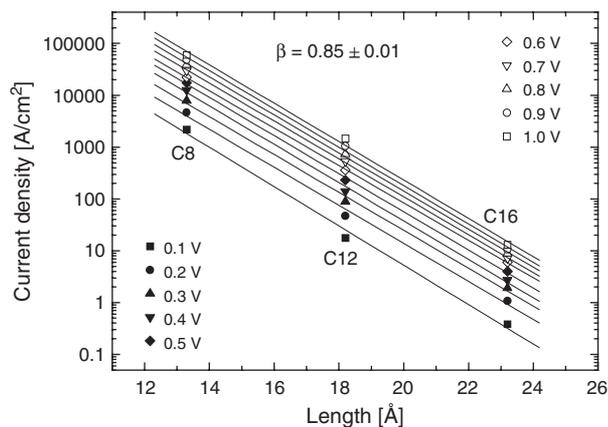
**Fig. 3.** Semilog plot of tunneling current densities of three different alkanethiol SAMs versus molecular length. The lines through the data points are exponential fittings.
