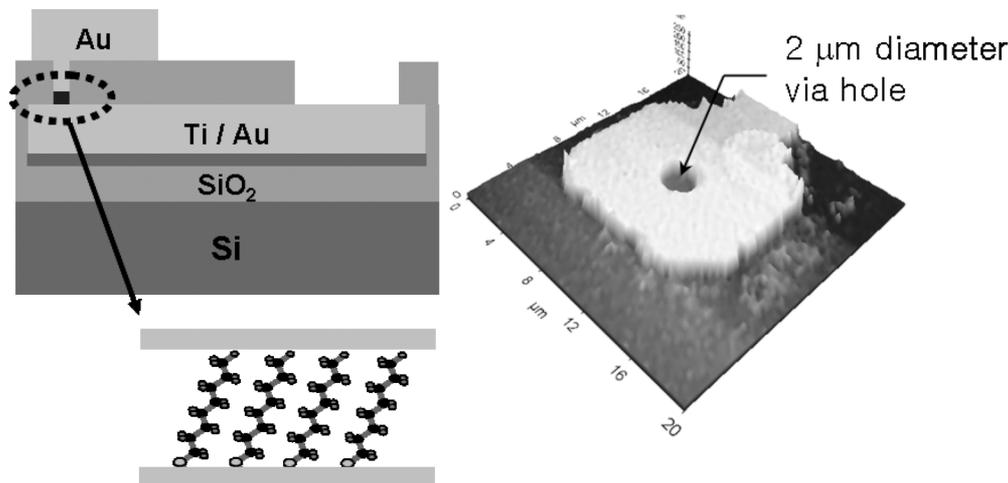
**Fig. 1.** Schematic of a micro-via hole structure and an AFM image of a single device. The typical junction is  $\sim 2 \mu\text{m}$  in diameter.
